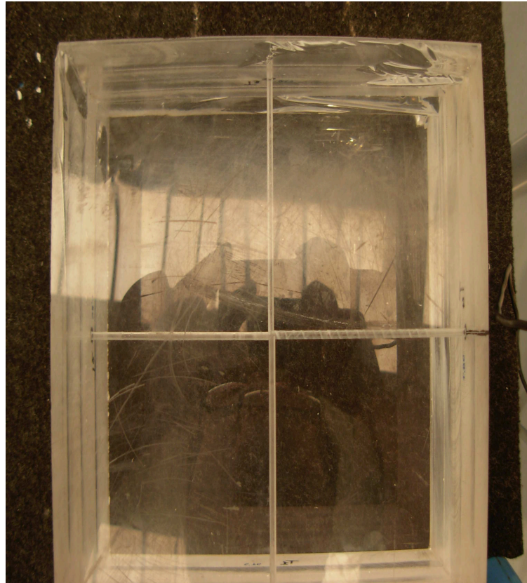
PMMA after drilling with holes for thermocouples
