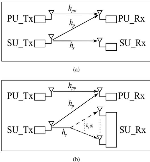
Figure 1. (a) A spectrum sharing channel model (b) Equivalent model adopting the broadcast approach.
